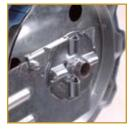
The Janus ratchet tensioning device supplied as standard equipment on our door offers a simpler method of tensioning, while more accurately fine tuning all the springs on the door at the same time. Eight different positions on the tension wheel allow one to perfectly balance the door every time. There are no pins required to hold the tension on the spring. You simply just click it.
