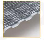
Insulation is made of a foil-backed, dual-layer polyethylene air-bubble insulation secured in place with a strong adhesive and joined by mylar film to provide an R value of 4 (top draft stop and side draft stops are also included). Model 1100l only.
