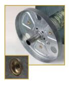
9 ½" diameter drums allow for lower headroom requirements. An enclosed barrel houses the dead axle assembly and protects the factory-lubricated springs from direct contact with environmental elements. The inherent strength provided by the spiral barrel minimizes axle deflection, providing smoother operation. Because the curtain is attached by screws and not seamed to the barrel, cost-effective replacement of either independent assembly is quick and easy.
