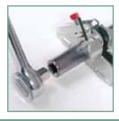
Convenient spring tension adjustment is accommodated by inserting a common 3/8" ratchet tool into the end of the drive shaft and rotating. Initial loading of the door tension can be easily accomplished with a ratchet without the difficulty of spinning the door. This innovation also allows the tension to be easily measured and managed with a torque wrench.
