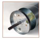
9-1/2" diameter drums allow for lower headroom requirements. An enclosed barrel houses the dead axle assembly and protects the factory lubricated springs from direct contact with environmental elements. The inherent strength provided by the spiral barrel minimizes axle deflection providing smoother operation. Because the curtain is attached by screws and not seamed to the barrel, replacement of either independent assembly is cost-effective, quick and easy.
