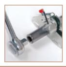
Convenient spring tension adjustment is accommodated by inserting a common 3/8" ratchet tool into the end of the drive shaft and rotating. Initial loading of the door tension can be easily accomplished with a ratchet without the difficulty of spinning the door. This innovation also allows the tension to be easily measured and managed with a torque wrench.
