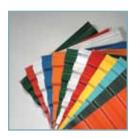
The 26 gauge corrugated door curtain is manufactured from full hard galvanized grade 80 steel and coated with Super Durable polyester paint that is backed by a 40 year film integrity and 25 year no-fade limited paint warranty. Available in sizes up to 18'0" x 18'0" and in over 20 different standard colors.
