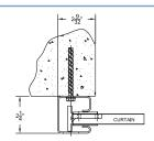
CONCRETE AND FILLED MASONRY BLOCK JAMBS (USING POWERS 1/4" x 3" WEDGE-BOLT)
