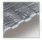
Insulation is made of a foil backed, dual layer of heavy-duty polyethylene air-bubble insulation secured in place with a strong adhesive and joined by mylar film to provide an R value of 4. (Top draft stop and side draft stop are also included.)
