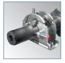
A cam-action spring tension holding device allows quick, easy and equal adjustment of the tension on all springs simultaneously from one end of the door. The cam tensioner bites into the axle helping to eliminate the unwanted spinning of the axle during the initial spring loading or adjustment process.
